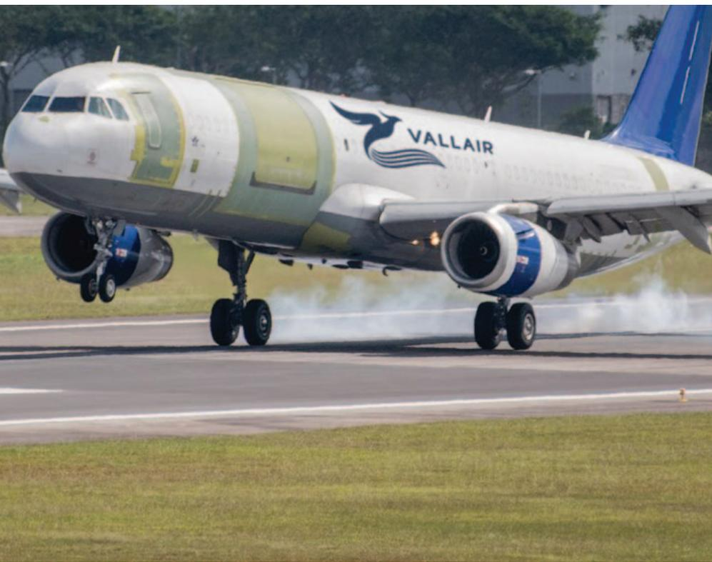
service it will typically carry no more than 23-24 tonnes or 50,706-52,911lbs. This is because the aircraft will be operating primarily in the lower-density express freight market. Increasing the A321PCF cargo capability above 27 tonnes or 59,525lbs will require more structure, cause higher OEWs and negatively impact the performance and operating costs," says Young.
